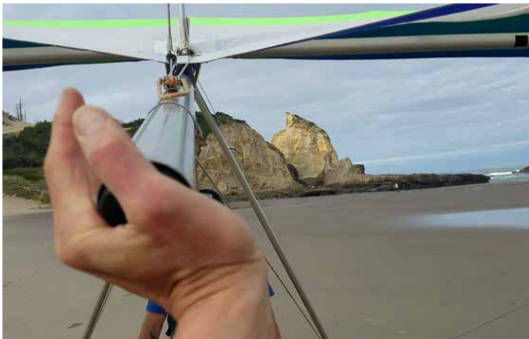
PHOTO 3 This is the proper way to hold the keel in a buddy carry; alternatively, you can use your shoulder to go hands-free.
