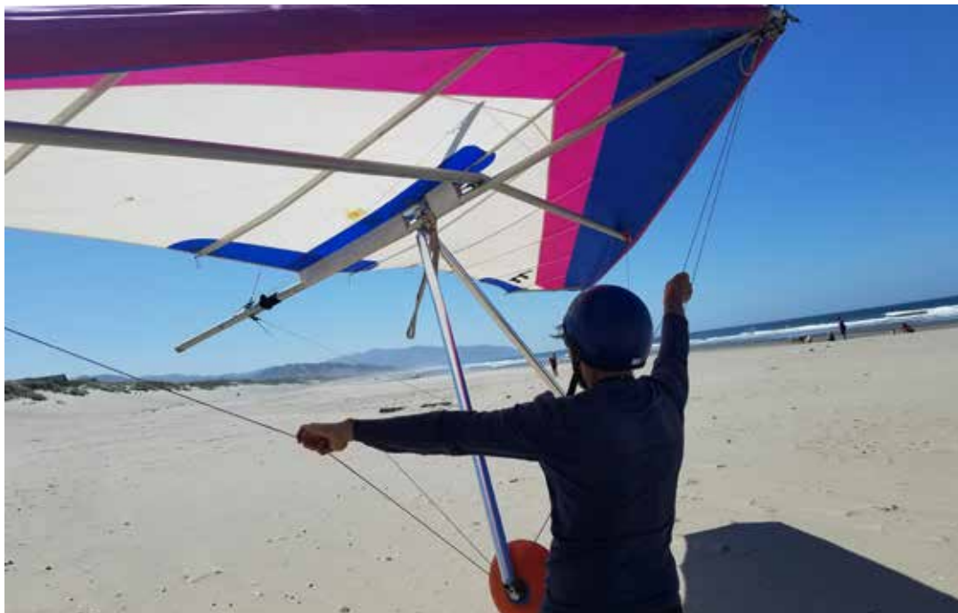
PHOTO 2 Hand placement on the side wire with body triangulation when the terrain lifts one wing. You are pushing down on the wire to keep the wings level.
