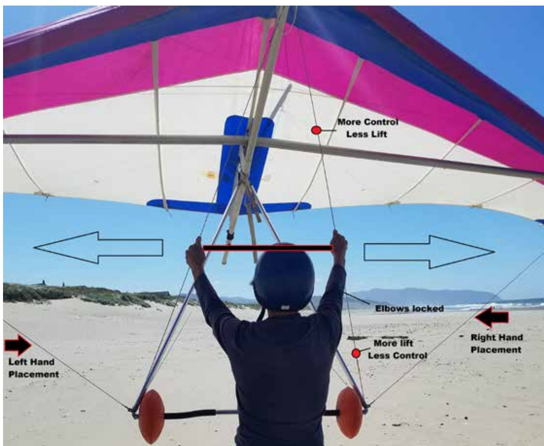
PHOTO 1 A useful technique for kiting hang gliders is to imagine there are rigid handcuffs attached to your wrists requiring simultaneous movement of both your left and right hands to yaw the glider slightly. The limiting arm is the one on the side where the wing is being lifted. If you let go of that side, you can get even more yaw and leveling. Here, advanced instructor John Matylonek demonstrates the basic kiting position on the beach at Pacific City, Oregon.
